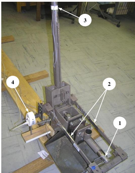
Fig. 4 Arrangement of the sensors: 1 - full bridge on the piston, 2 - two gauges on each of the connecting rods, 3 - 1/2 bridge on the lever and 4 - the position angle digital sensor.
