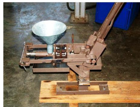
Fig. 1 Schematic illustration of the ram press machine
