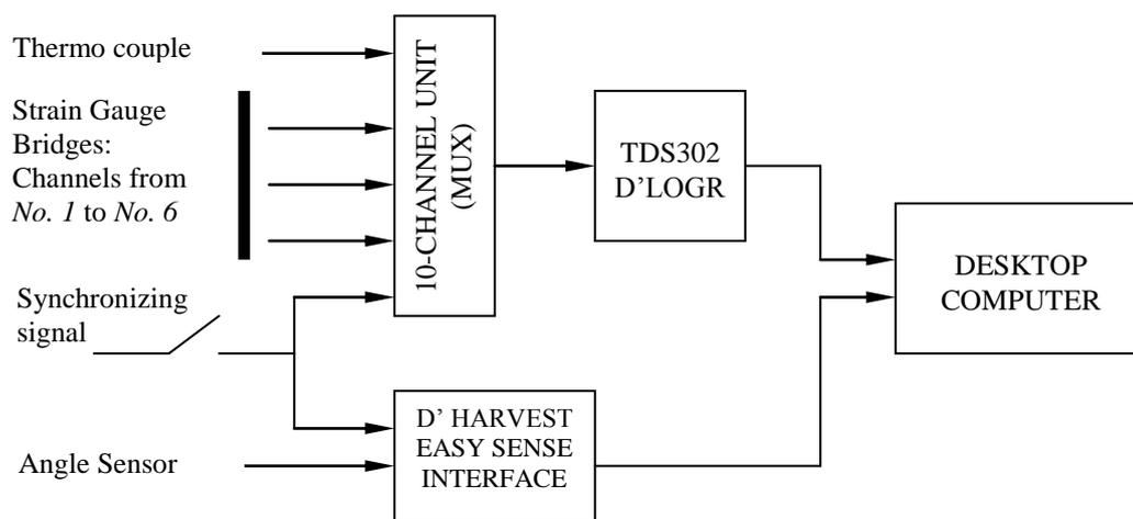
Fig. 7 Block diagram of the Instrument System for the forces and moments measurements.
