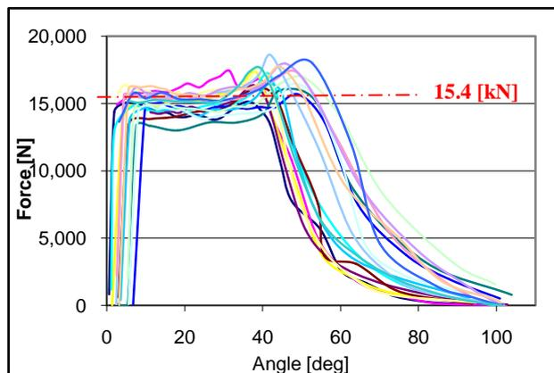
Fig. 10 Tension forces on the connecting rods
