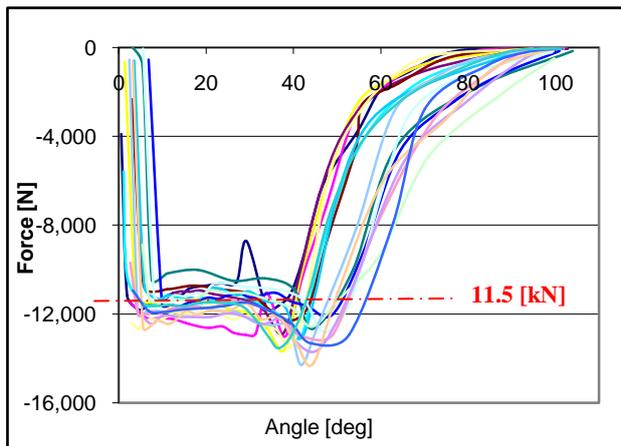
Fig. 8 Variable compressive forces on the piston
