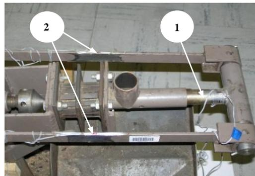
Fig. 6 Full bridge electrical strain gauges bonded at the end of piston (ram) - 1 and two strain gauges attached to each of the connecting rods - 2.
