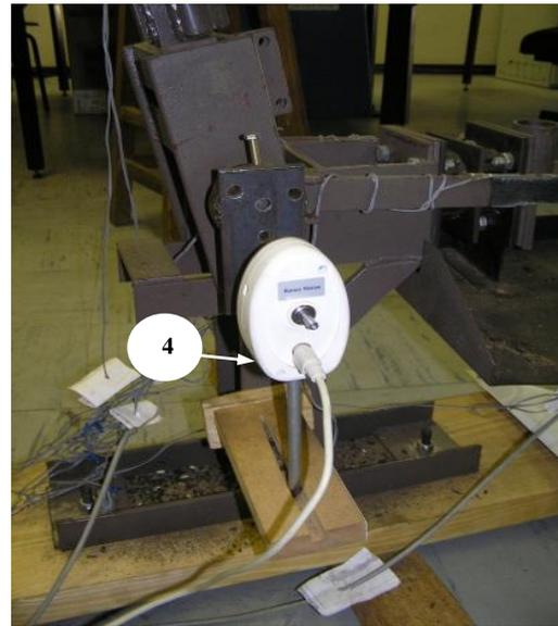
Fig. 5 Position angle digital sensor – 4.
