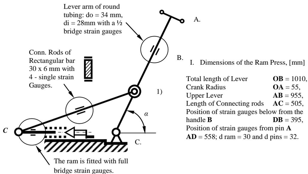
Fig. 3 Positions of strain gauges as installed on the BP30 ram press machine
