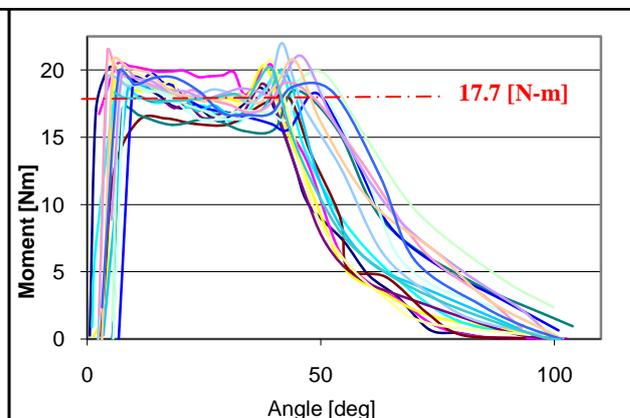
Fig. 11 Bending moments on the connecting rods
